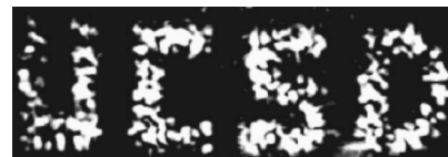
Fig. 3. Far-field reconstruction for 1.55 \mu\text{m} . Speckle noise can be eliminated by replicating the phase function several times along the element plane.
