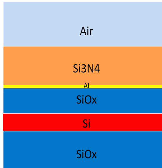
Figure.8 Illustration of a multiple slab IMI structure with an infinite slabs SiO x , silicon slab, SiO x slab, Al slab, Si 3 N 4 slab and air
