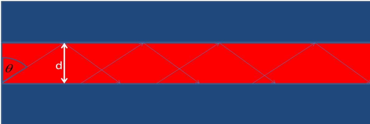
Figure.3 Illustration of a symmetrical three layer slabs waveguide with two wave fronts propagating in it.
